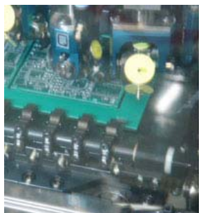
Photo of the board in the pick and place machine.
